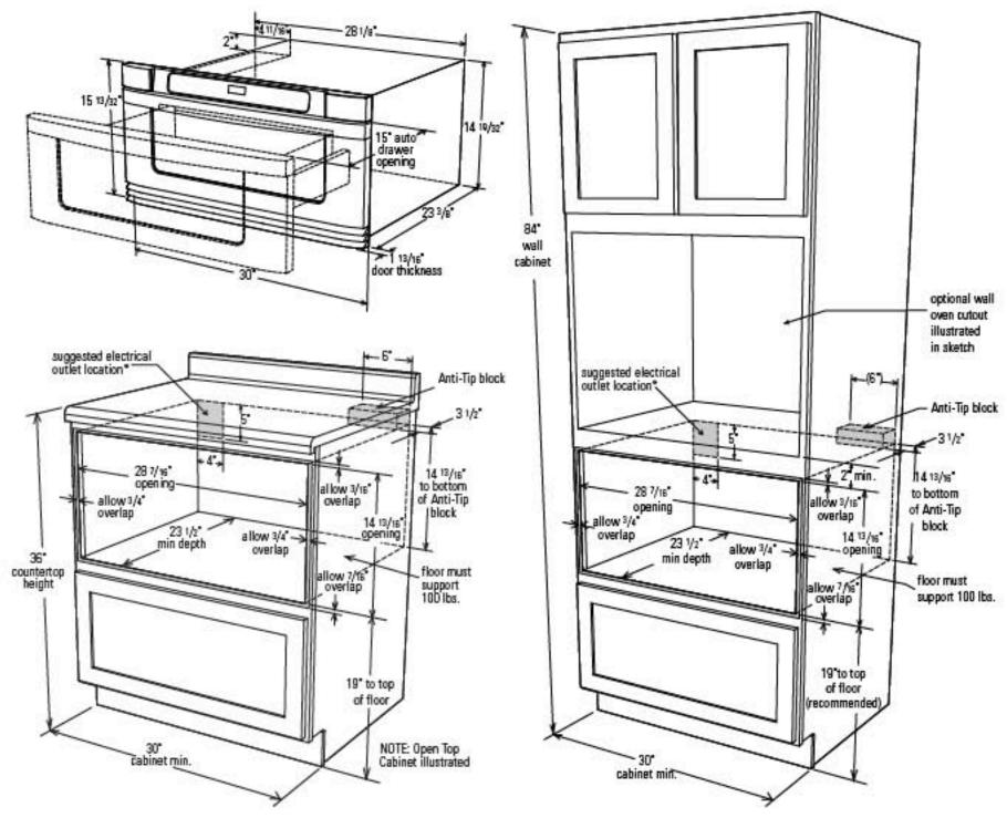
This Microwave Drawer can be installed below any electric or gas wall oven.
