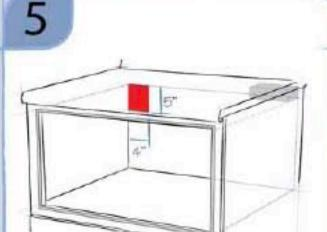
Place electrical outlet in upperback left side of opening. Electrical outlet can also be placed in an adjacent cabinet. Always check electrical codes for requirements. Proceed to Installation Instructions to install Drawer into cabinet.
