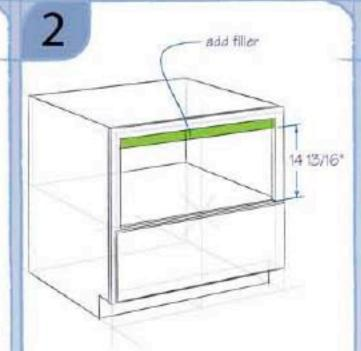
Add horizontal filler to the top of the opening. Height of opening should be 14 13/16".
