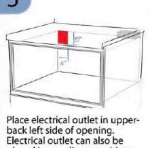
Place electrical outlet in upperback left side of opening. Electrical outlet can also be placed in an adjacent cabinet. Always check electrical codes for requirements. Proceed to Installation Instructions to install Drawer into cabinet.
