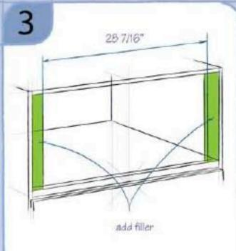
Add vertical fillers to the opening width. The width of the opening should be 28 7/16".
