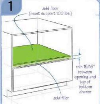
Remove top two drawers and slides. Add filler and support surface. Must support 100 lbs.
