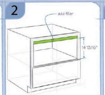
Add horizontal filler to the top of the opening. Height of opening should be 14 13/16".
