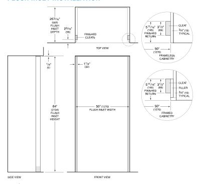
NOTE:  $3^{1}/2^{n}$  (89) finished returns and shaded areas will be visible and should be finished to match cabinetry. Shaded line represents profile of unit with  $3^{1}/4^{n}$  (19) panel.
