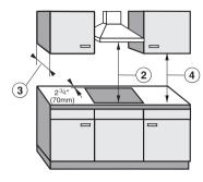
As a general rule there must be at least 30" (760 mm), ②, between the top of the appliance and any cabinet above it. The maximum depth, ③, of cabinets installed above a cooktop must not exceed 13" (330 mm). The minimum distance of combustible surfaces located above and to the sides of the cooktop, ④, is 18" (457 mm).
