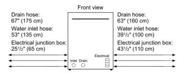
All connections at the rear of the appliance. Extensions for drain hose available as accessory. Electrical cable for outlet connection (3 pin plug) available as accessory.
