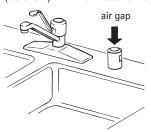
that the drain hose either be looped up and securely fastened to the underside of the counter, or be connected to
