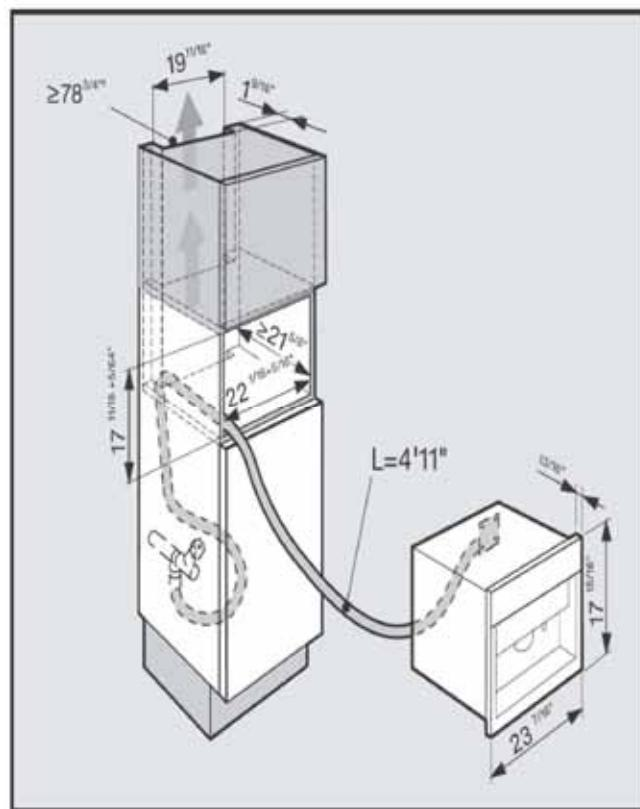
**PLEASE NOTE:** The vent cut out must only be at the top of the niche to prevent condensation inside the door and inner components that the customer can see when opening the door.
