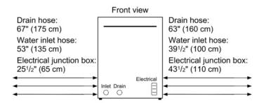
All connections at the rear of the appliance. Extensions for drain hose available as accessory. Electrical cable for outlet connection (3 pin plug) available as accessory.
