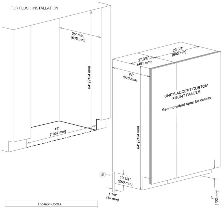
E- power cord for refrigeration unit- 5 foot- NEMA 5-15 molded plug power supply connects lower left rear of units
