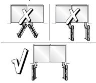
If the appliances are installed directly next to each other (without a partition), they need to be attached together. A heating mat must also be installed. This will help avoid condensation and prevent damages.
