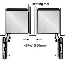
In this case, you will only need the heating mat from the "Merging kit" to avoid condenstaion and prevent damages.
