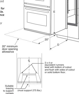
Cutout depth Cutout width 23-1/2" MIN. 25" MIN. Junction box 25-1/4" MAX. (Junction box may be located В junction box Cutout height 41-1/8" MĬN. 41-1/4" MAX. Recommended minimum cutout location from the floor 21-5/8"
