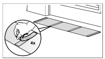
3. Fit the toe kick panel to the base panel and press firmly into place.
