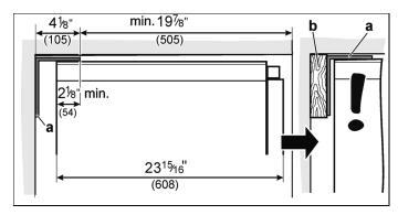
The length of the plank should correspond to the width of the installation enclosure!
