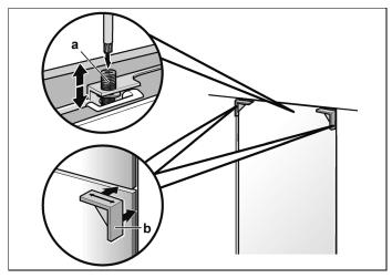
3. Transfer the middle drill holes along the outer edge of the appliance door to the door panel and mark.
